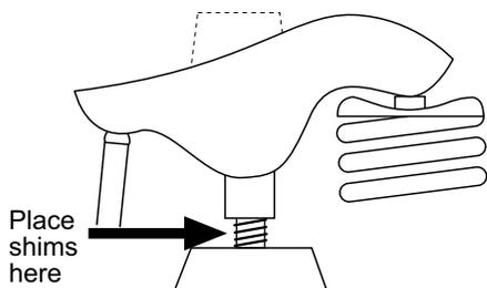
Figure 1. Typical installation for V-8 engines such as Olds V-8, some AMC V-8 and 6 cylinder and '81 and up 151 cu. in. Pontiac 4 cylinder engines.
