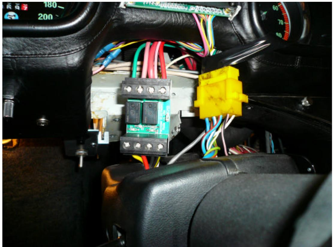
Typical position of the ISB after replacement of original connector without modifying wire length Image 5
