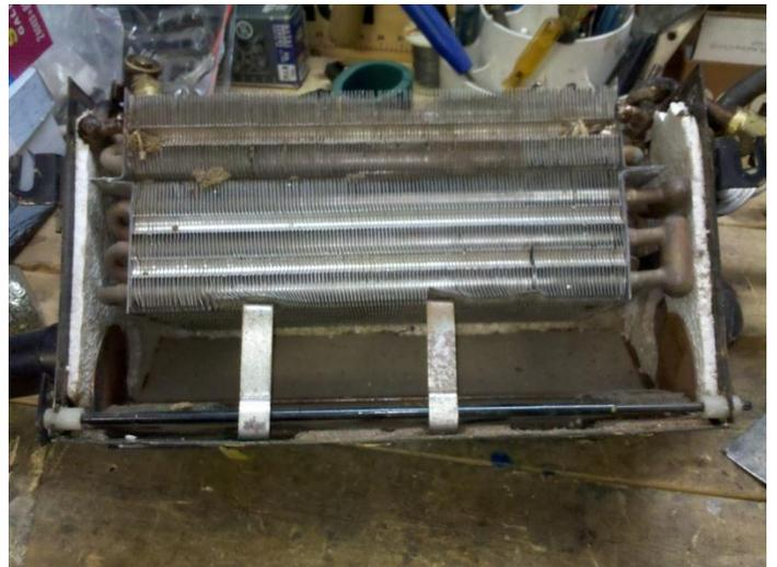
8. If you are replacing the evaporator, fit it in the heater box. The feed lines bend some but you do not want to bend them much or too often as they will break.
