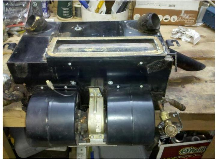
With the heater box out of the car, you can clean all the area back there, reroute accessory and stereo wire, and even fix any rust that may reside around the fresh air vent.
